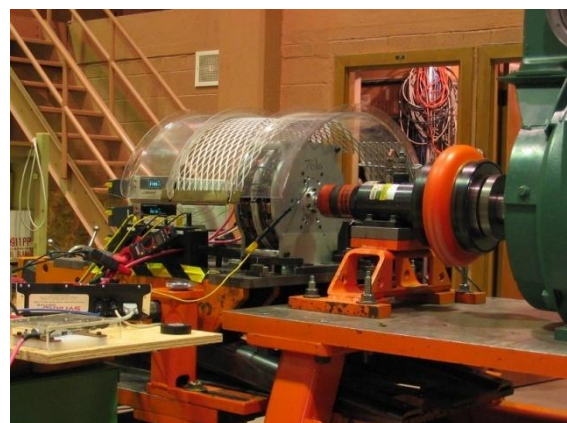
Figure 8: Proof of Concept (PoC) motor under load test
